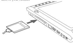
Figure 2-3 Installing a PC Card
